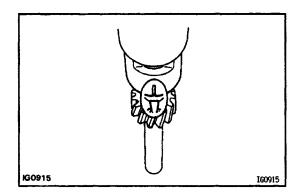
(b) Align the protrusion on the driven gear with the groove of the distributor housing.
