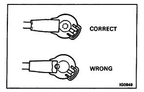
NOTICE: Check that the holder is correctly installed to the grommet and distributor cap as shown in the illustration.
