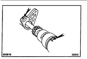
(c) Insert the distributor, aligning the groove of the distributor housing with the groove on the No.4 camshaft bearing cap.
